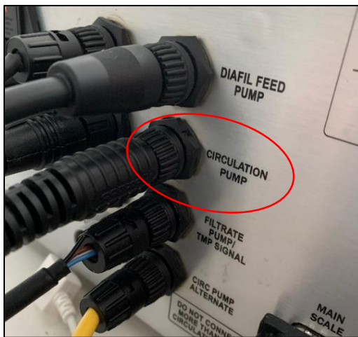
Figure 3/4: PDKT-LFC-TFF interface cable connected to PendoTECH TFF and Levitronix PuraLev Flow Controller.
