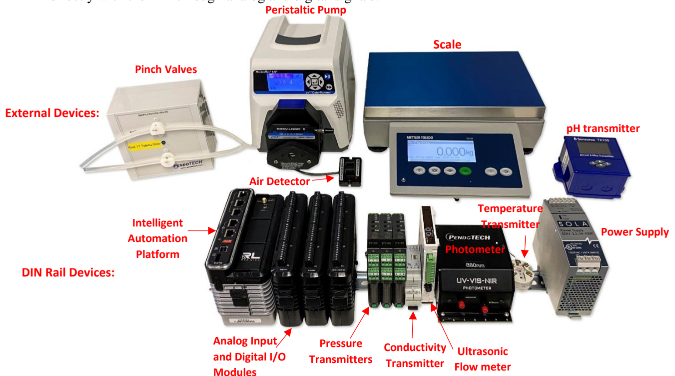
Figure 4: Annotated picture of physical setup of PendoTECH’s Industrial Single Use System
