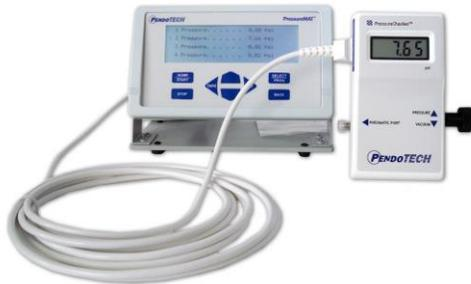
This has an upper test limit of 10 psi which is the PressureChecker limit because it is designed for high resolution readings and the limit of the calibrated internal reference pressure transducer (that reads on the LCD).
