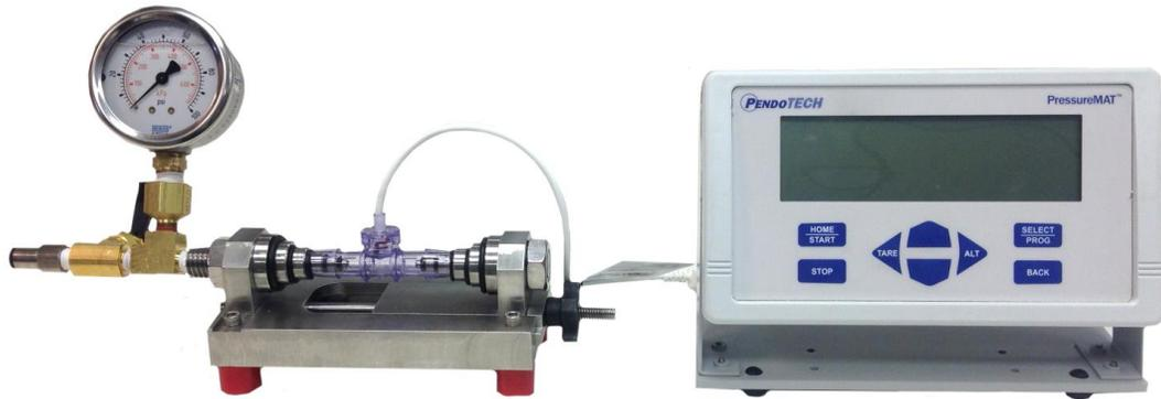
Because this involves testing the sensor only, it would be most useful for sensor qualification testing or post-use testing of a sensor removed from a disposable assembly.
