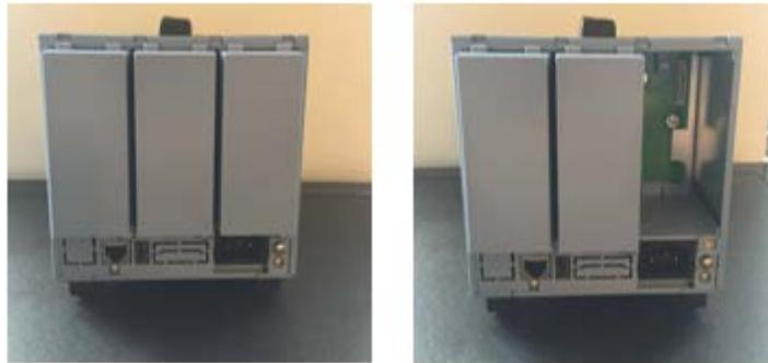
2. Remove cover on analog input module to access screw terminals. Cover is held in place by a screen on the bottom and clips on top. The cover can be replaced once all connections have been made with PMAT.
