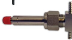
Low hold-up volume cell shown with 1/8inch hose-barb inlet and outlet and micro coupler installed. Available with 1cm and 0.5cm path length.
