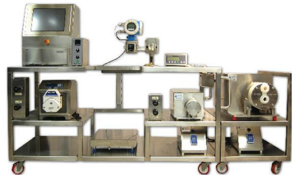
*Pilot cart shown with push-up cart with larger pump demonstrates system flexibility that is required in Pilot environments.*
