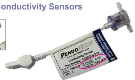
The system measures conductivity via the PendoTECH Single Use Conductivity Sensor which is also robust enough for cleaning and extensive reuse. The sensors are available in a range of sizes. All sensors have a pre-determined cell constant that is printed on their tag which is entered into the software. Temperature compensation performs normalization to 25°C and have a measurement range of 0 to 100mS.
