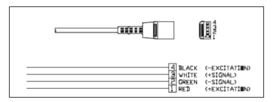
The reusable cable connected to the transmitter/control system has five wires- four are illustrated in the image, and the fifth is a cable shield.
