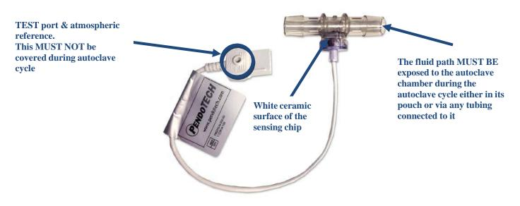
^ The TEST port can be used to non-invasively test functioning of the pressure sensors and its monitor pre- and post-use with the PendoTECH PressureChecker<sup>TM</sup>
