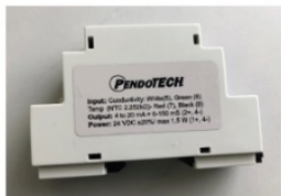
Wiring information conveniently printed on the unit
