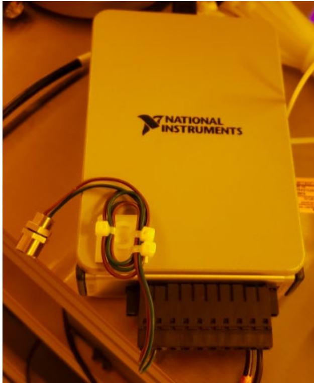
Figure 1 PendoTECH connector to NI 9265 Box
