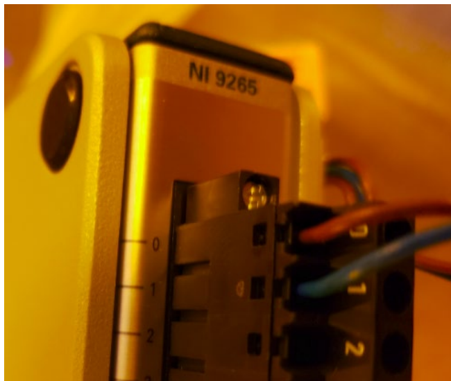
Figure 1. Connector wire connections to NI 9265 Box
