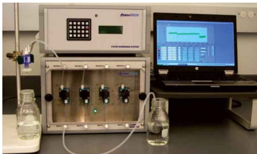
Photo 1: PendoTECH normal-flow filter screening system
