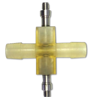
Optical Couplers Installed to Flow Cell
