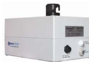
Figure 6. One normally open pneumatic pinch valve with air inlet on box and power supplied to solenoid valve in the box via connector on rear for remote control of valve
