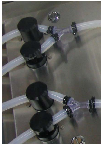
FIGURE 3. Normally Closed Pneumatic Pinch Valves Mounted in a Stainless Steel Box
