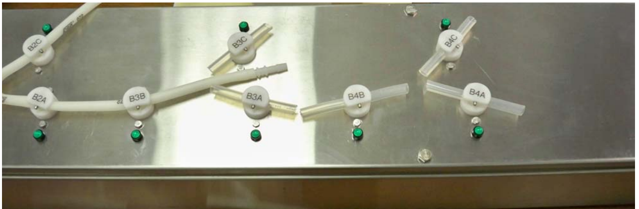
FIGURE 2. Normally Closed Electric Pinch Valves Mounted in a Stainless Steel Box with LED indicators
