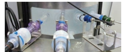
Non-invasive probe shown next to traditional probes in single use bioreactor
