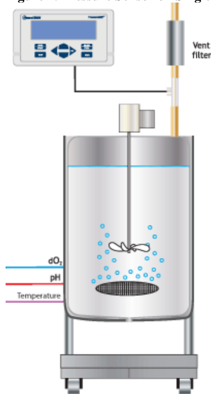
Figure 1. Pressure Sensor on Single Use Bioreactor
